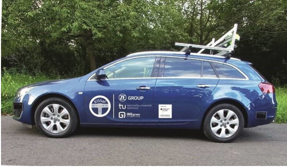
Figure 1 The KISSaF measurement vehicle equipped with radars, camera and lidars.
